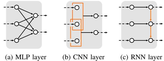
Figure 2: Overview of network architectures in security: Multilayer perceptrons (MLP), convolutional neural networks (CNN), and recurrent neural networks (RNN).
